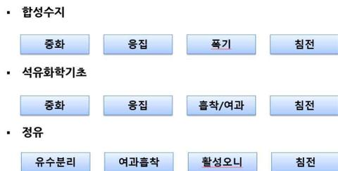
Fig. 3 Wastewater treatment process by industry.
